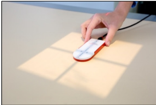
Photo 1: With Nomex Multimeters, there is no need for additional alignment along the tube axis, which accelerates and simplifies measurement setup
