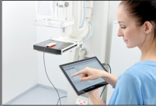
Photo 2: The Nomex Multimeters are easily connected to and operated using a PC or tablet via mini USB port and plug-and-play without any additional accessories, as shown in the photo of the NOMEX Multimeter MAM on a mammography device
